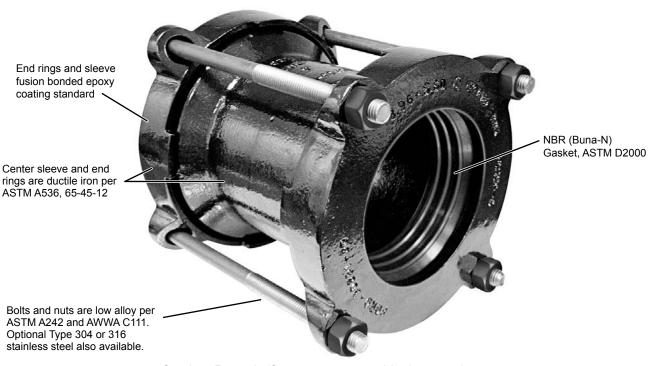
Caution: Restrain if necessary to provide thrust resistance. Flexible couplings do not prevent axial pipe movement.
