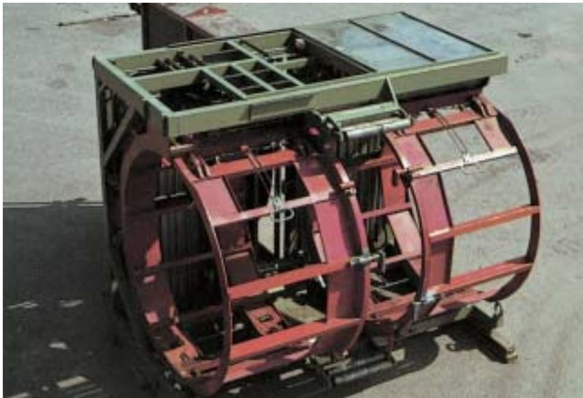
*Machine de fusion 63 po KWH PIPE*
