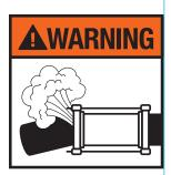
THIS PRODUCT DOES NOT RESTRAIN PIPE MOVEMENT. Proper anchoring is required to prevent pipe pullout. Failure to anchor or improper anchoring can result in dangerous pipe content escape, property damage, serious injury, or death. Read the product installation instructions prior to installing this product.
